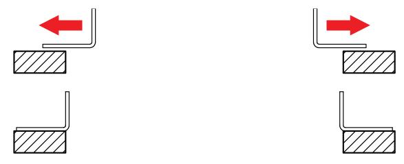
Step 2: Screw the plaster frame to the mounting clip. The drywall should be in between the plaster frame flange and mounting clips.
