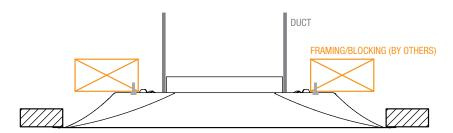
Step 7: When the back pan is securely fastened, reattach the diffuser's inner core assembly to the frame (see page 6).
