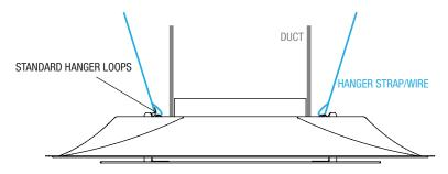
Step 3: Attach and secure the hanger straps or wires to the structure.
