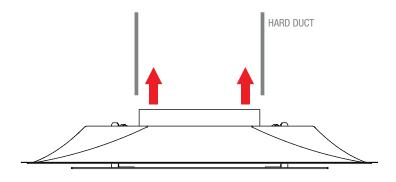
**Step 3:** Screw the back pan's inlet to the hard duct work.
