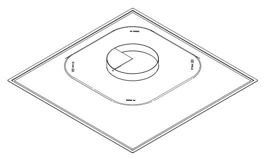
**Step 2:** Screw the sectorizing baffles directly to the round inlet.
