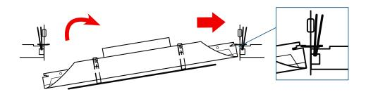
Step 4: Make sure the diffuser is centered and secure the duct to the inlet of the diffuser. Note Access through adjacent panel required.
