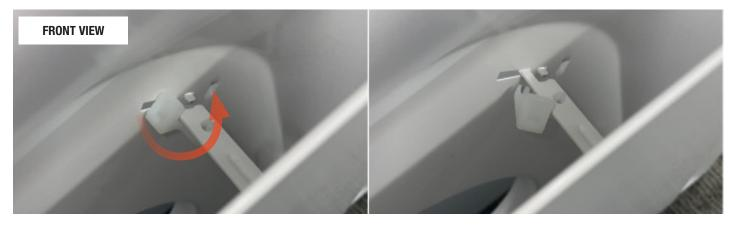
Step 2: Once unclipped, push the inner core slightly and rotate counter clockwise until the hook of the mounting legs comes loose.
