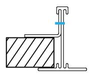
**Step 3:** Lay the diffuser on the plaster frame.
