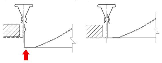
Step 3: Attach and secure the duct to diffuser's inlet.
