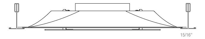
**Step 2:** Mount and secure the duct to the diffuser's inlet.
